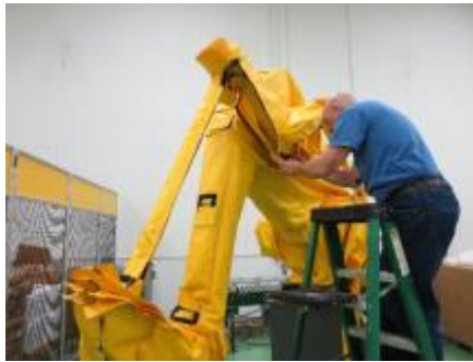
Starting Near J4, Install the Fwd Link/Boomerang. Move Toward J2
