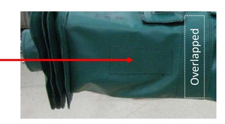
Install zip tie (or clamp) around the cuff at tool flange. Be certain to clamp on the non-rotating casting of the upper-arm and NOT the rotating tool flange as the cover will twist if clamped to the rotating tool-flange.
