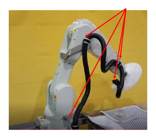
Depending on your specific dress-pack, spacers may be required to create sufficient stand-off between the bracketry and the Robosuit®.
