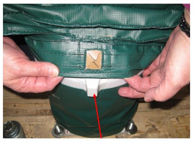
Align the finger and window to properly orient the lower-arm cover.
