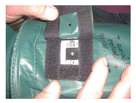
Open the flat Velcro access panel near joint-4.
