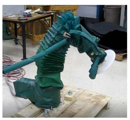
Reinstall cables/conduit/dress packs at this time. If you specified protective cable wrap, install it at this time.
