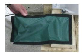
If the robot is mounted inverted: The flat panel must be installed as it will be used to hold the base cover in proper position while the robot operates inverted.
