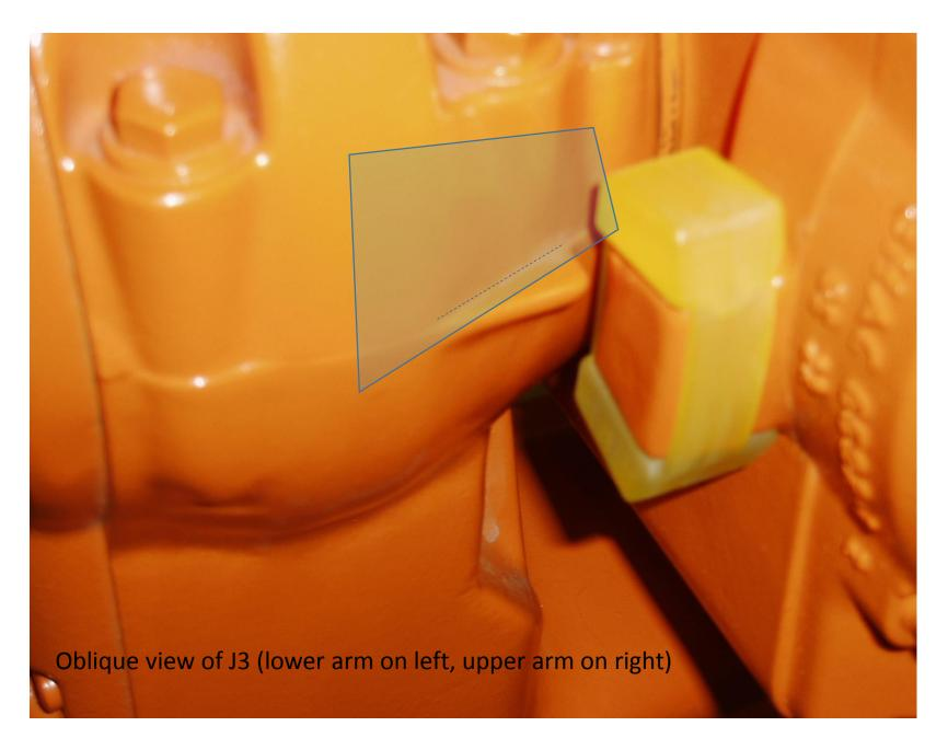
Approximate "grind" angle is parallel to the indexer cast line at the lower arm interface.
