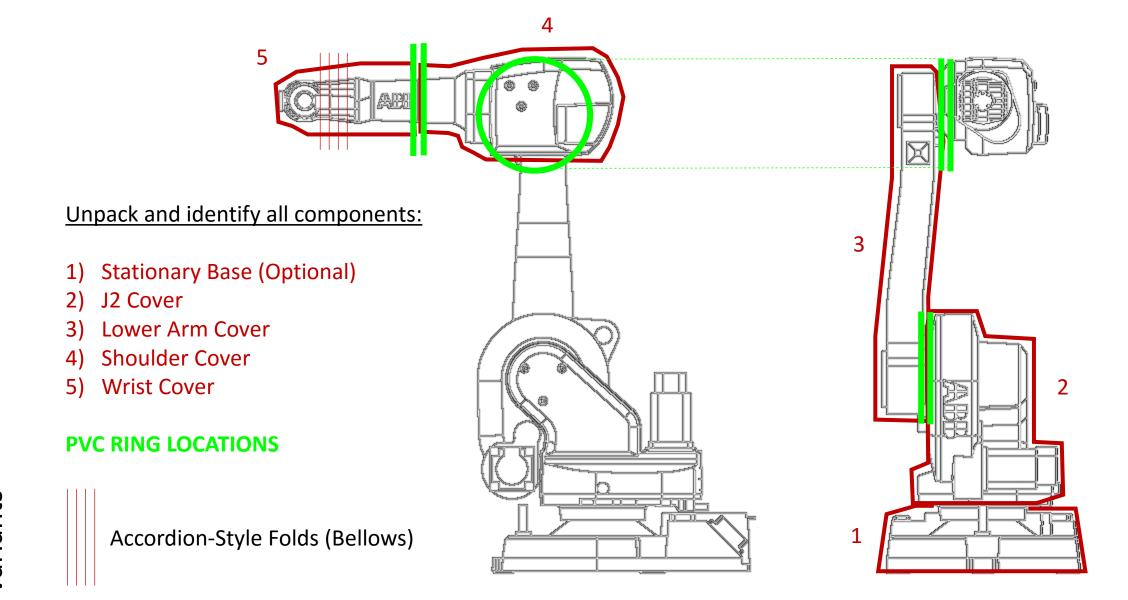
PRIOR TO INSTALLING THE ROBOSUIT<sup>®</sup>, CLEAN THE ROBOT SURFACE IF THE ROBOT HAS BEEN IN OPERATION WITHOUT ANY EFFECTIVE PROTECTION. DISCONNECT ANYTHING THAT WILL INTERFERE WITH INSTALLATION. NORMALLY, END-OF-ARM TOOLING DOESN'T INTERFERE IF THE ROBOT'S FLANGE IS FACE-OUT. IF POSSIBLE, PLACE THE ROBOT IN ITS SYNC ALIGNED (HOME) POSITION.
