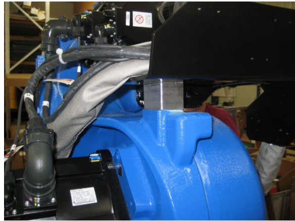
Photo-14: Insert aluminum block and M6x50 bolts (supplied)
