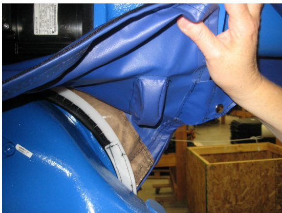
Photo-29: Bump Stop pocket (fit)
