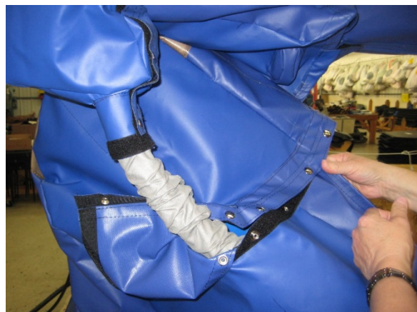
Photo-42: Close seams along top of arm
