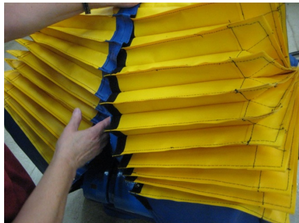
Photo-46: Align/Close Velcro seams along each bellow-fold
