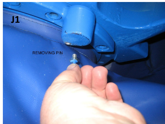
Photo-2: Remove pin from hard-stop on lower-arm (at J1)
