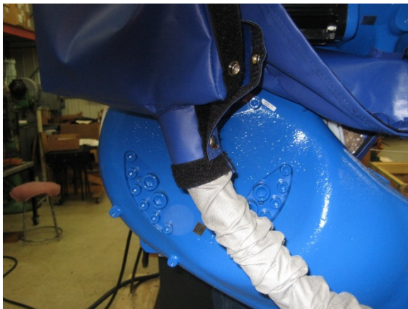
Photo-27: Work across shoulder closing seams/cable cuffs
