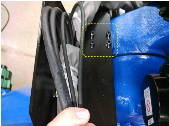
Photo-13: Remove the (Qty-4) M6x20 cap-head bolts
