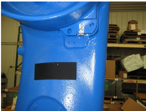
Photo-9: Apply 2"x4" Velcro HOOK tape to Lower Arm
