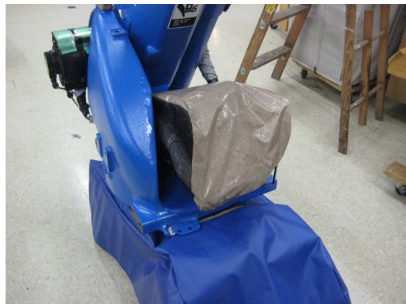
Photo-16: J1 servo motor cover
