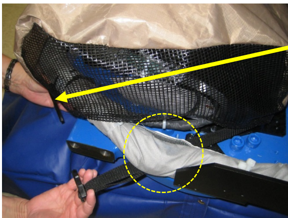
Photo-17: Strap routed underneath control cable bundle
