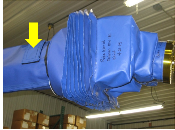
Photo-50: Velcro access panel locations
