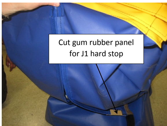
Photo-47: Cut gum rubber. Velcro band over base collar
