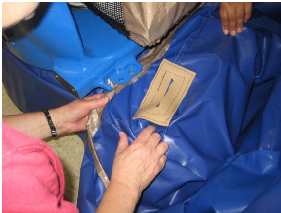
Photo-39: Mark the gum-rubber panel and cut
