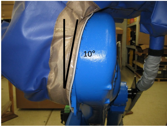
Photo-25: Upper Arm at J3. Note 10-degree deflection
