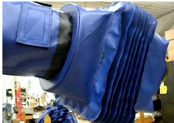
Photo-34: Wrist ring overlaps torque tube ring
