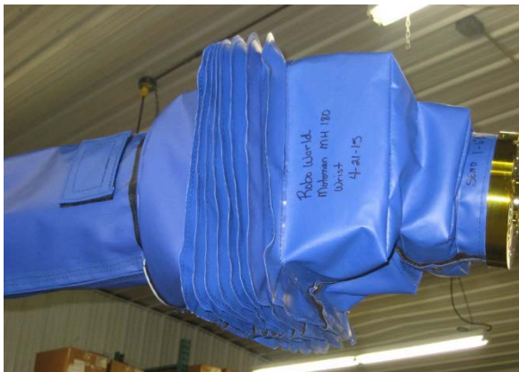
Photo-33: Zipper torque tube sleeve closed and install wrist
