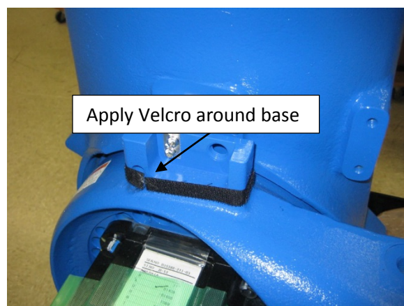
Photo-6: Apply 3/4" Velcro HOOK tape to J2 synch casting
