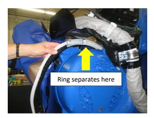
Photo-23: Separate the PVC ring and install as shown
