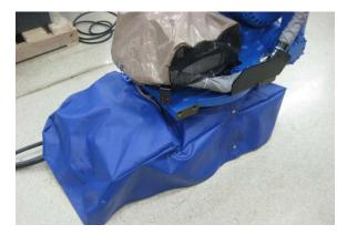
Photo-19: Stationary base cover (shown installed)
