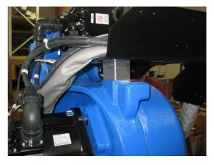
Photo-14: Insert aluminum block and M6x50 bolts (supplied)
