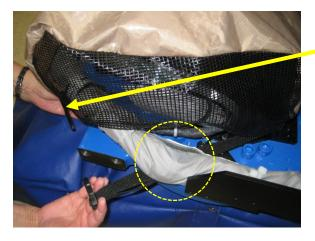
Photo-17: Strap routed underneath control cable bundle
