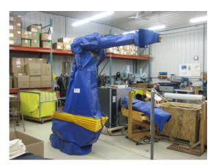
Photo-48: Installed MH225 Robosuit®
