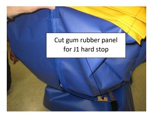
Photo-47: Cut gum rubber. Velcro band over base collar
