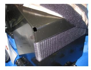
Photo-10: Apply 2" Velcro HOOK tape along J1 motor cover
