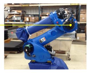
Photo-22: Begin Upper-Arm installation on this side of robot
