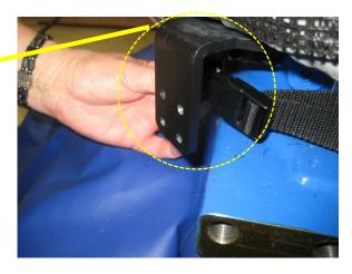
Photo-18: Route the strap under the mounting bracket
