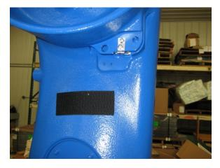
Photo-9: Apply 2"x4" Velcro HOOK tape to Lower Arm
