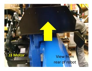
Photo-12: Cable tray atop J3 must be elevated before proceeding
