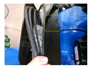
Photo-13: Remove the (Qty-4) M6x20 cap-head bolts
