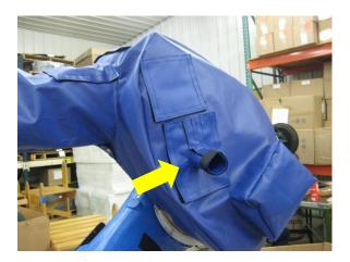
Photo-52: Cabling/Hose gooseneck access panel
