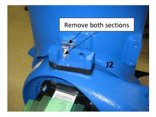
Photo-3: Remove both sections of synch markers at J2
