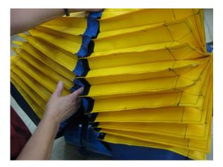
Photo-46: Align/Close Velcro seams along each bellow-fold
