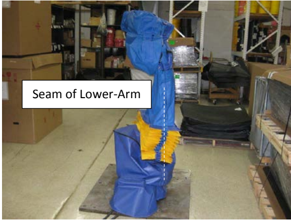
Photo-7, Orient Seam to the rear of arm
