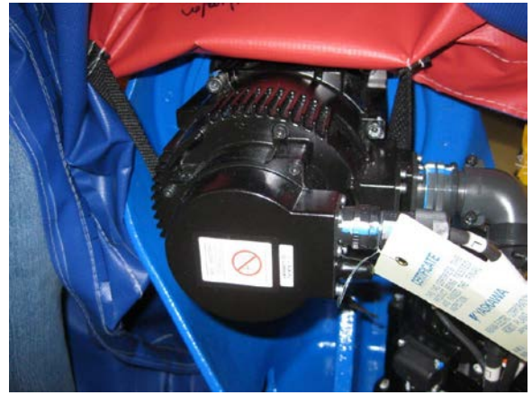
Photo-8, Secure the belt underneath the J2 motor
