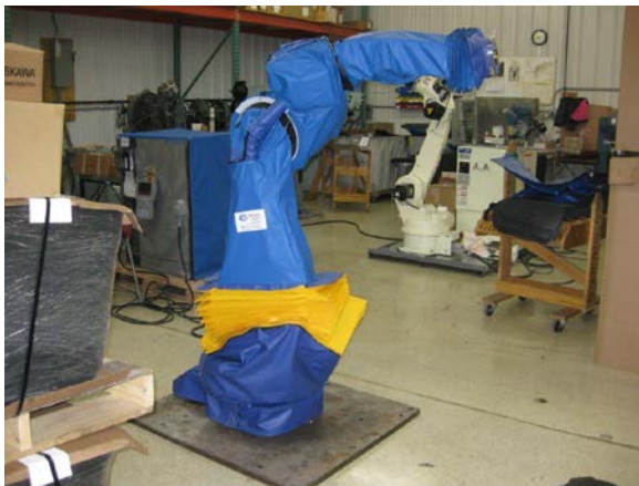
Photo-9, Note "relaxed" position of bellows
