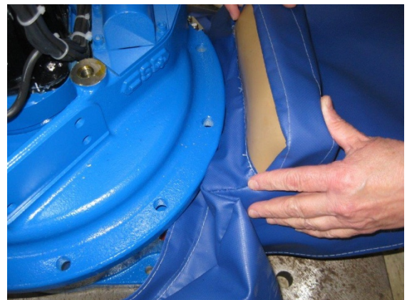
Photo-4, Orient Stationary base so gum-rubber faces robot
