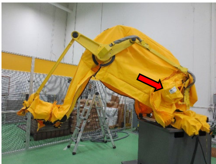
(Main) Arms Covered. Note: Boomerang, Ring (J3) and J2 motor Pocket
