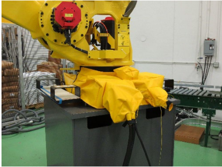
Installation of Stationary Base Cover Note: Pedestal Cover not shown
