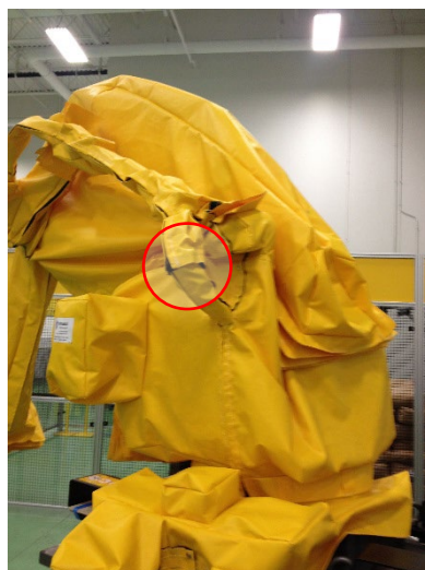
J2 Detail Note Cuff overlap at Link Arm.
