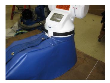
4. Install the lower arm cover (largest piece). Slide this section over the robot. Mate the Velcro to the upper-section of Velcro shown in the second image below.
