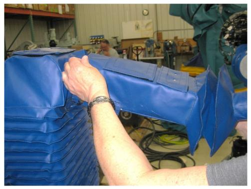
6. Install the clamp at the tool flange as shown below. Be certain to clamp on the <u>non-rotating</u> <u>casting</u> of the T-axis.
