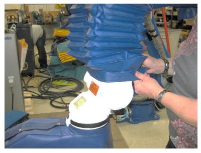
5. Install the upper arm/wrist. Orient the cover so that the Velcro panels are positioned atop the pneumatic connections. Overlap the lower arm cover cuff at R-axis as shown in second image below.
