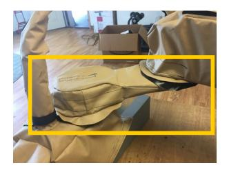
3. INSTALL THE UPPER ARM COVER. IT FEATURES TWO BELLOWED SECTIONS FOR THE QUILL. NOTE THAT A PEEL & STICK ADHESIVE VELCRO PAD IS AFFIXED TO THE INSIDE OF THE COVER. YOU MAY REMOVE AND INSTALL THIS SECTION OF VELCRO ADHESIVE PRIOR TO INSTALLATION, OR ONCE THE COVER IS LOOSELY IN POSITION, YOU MAY REMOVE THE ADHESIVE BACKING PAPER FROM THE VELCRO PAD AND ADHERE TO THE ROBOT CASTING.
