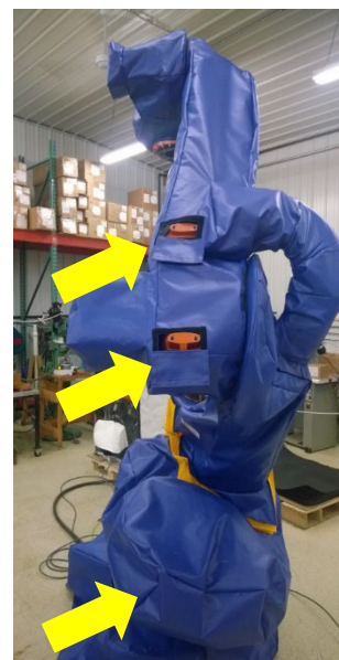
Photo-27: Hardware mounting access panel
