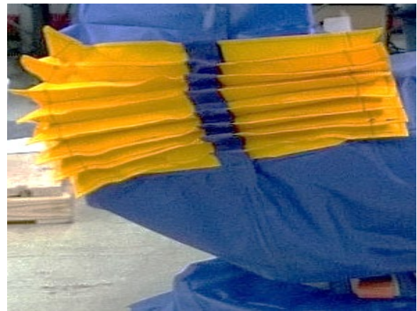
Photo-25: Close Velcro seams on bellows. Close remaining zipper
