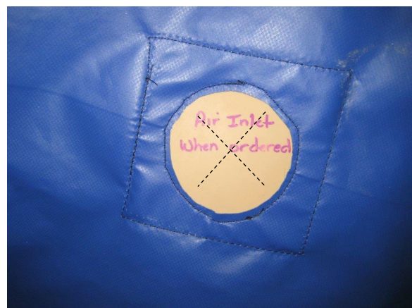
Photo-21: (Option) Cut the gum rubber pressurization port
