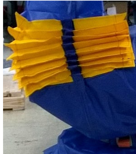
Photo-23: Close the bellows and leave bottom un-zipped
