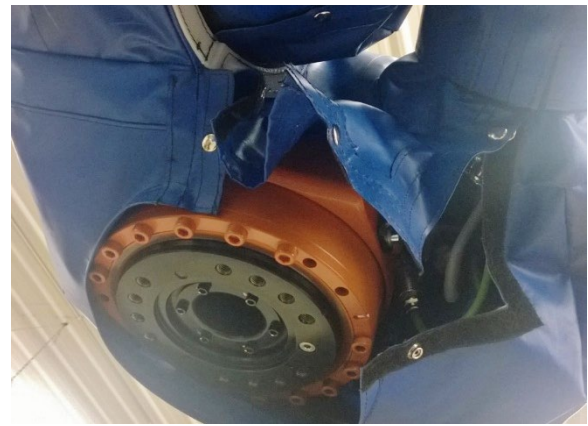
Photo-17: Wrap tool flange and secure all seams/snaps
