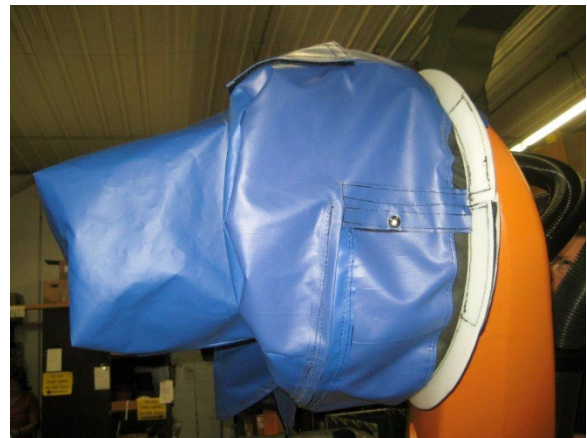
Photo-13: Properly installed shoulder (Ring J3)
